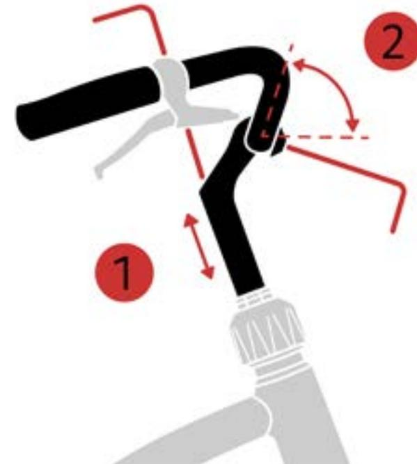
**Step 2:** To adjust the angle of the handlebar, loosen the allen bolts of the front plate until you can move the handle bar freely. Once you've found your preferred bar angle, tighten the bolt.
