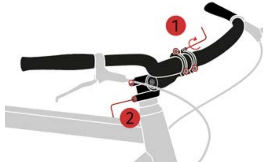
**Step 2:** Next, align the handlebars so that they are straight and perpendicular to the frame. Then, tighten the handlebar stem to the front fork, using the 4mm allen key.
