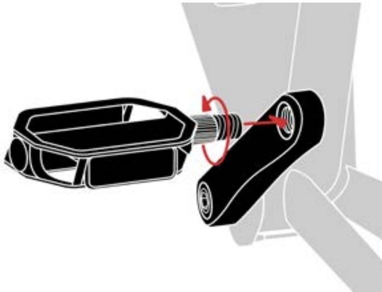
RIGHT pedal: This pedal has no indented lines and is smooth in between the pedal and thread
